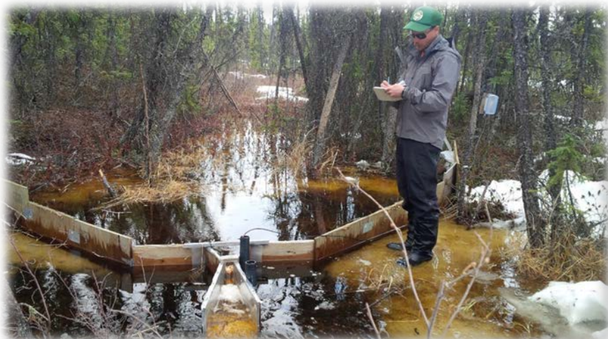
Ryan measuring streamflow from a flume box in SCRB, NWT.
